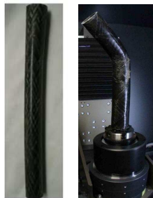
banded fibre reinforced tube (thermoplastic matrix)
