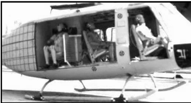
Full scale drop test of Bell UH-1D (Helisafe TA), Upon impact (left) and after (right)
