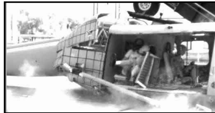
Full scale drop test of Bell UH-1D (Helisafe TA), Upon impact (left) and after (right)
