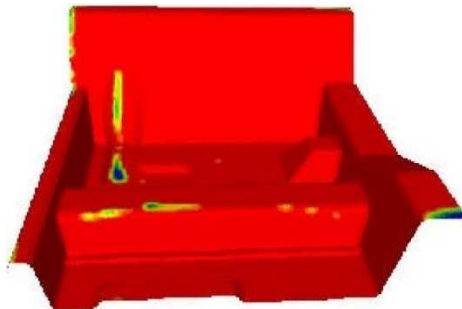
Mold filled to 100%
