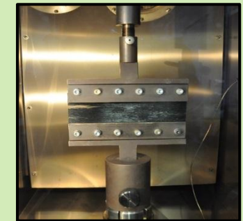
Tensile test cross fibre direction
