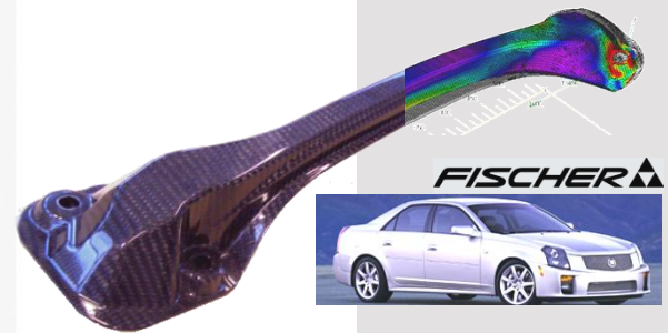
RTM – CFK – strut bar
