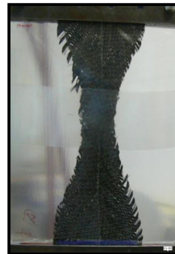
Bias Extension Test using a Single Ply with the Stitching running from Clamp to Clamp
