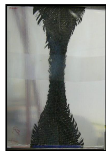
Bias Extension Test using a Single Ply with the Stitching running from Clamp to Clamp
