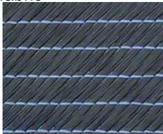
Typical Stackup : Non-crimped fabric
