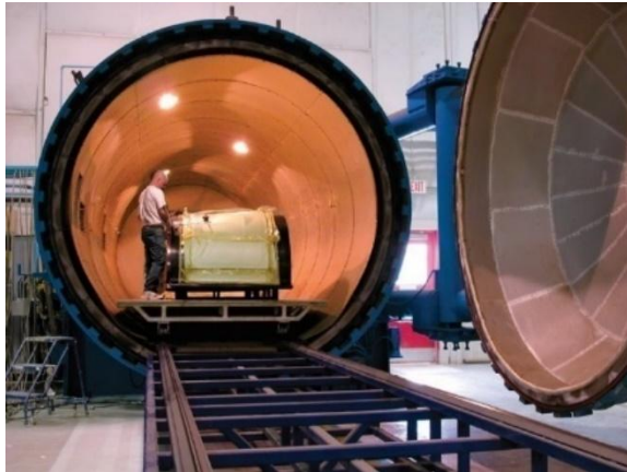
A composite component is positioned within the autoclave at American Airlines' composite repair shop, at the airline's Tulsa, Oklahoma, maintenance complex. Credit: American Airlines
