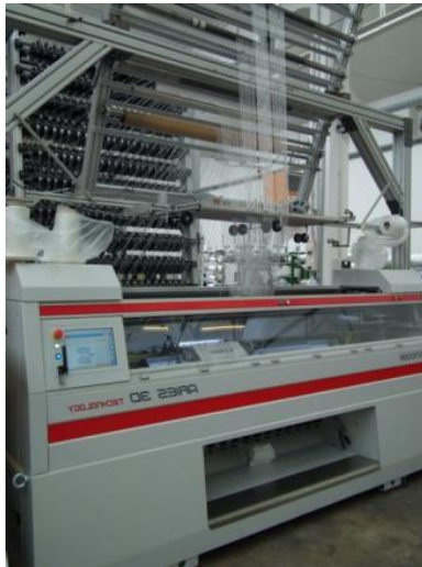
automated process, Steiger „Aries 3D“ flat bed knitting machine
